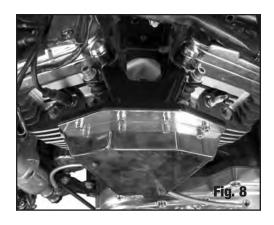
8. Install high flow petcock or high flow dual feed petcock to fuel tank. Follow instructions supplied with petcock (not supplied in kit). If you are using a single feed high flow petcock, you will need to install a "T" inline to supply the carburetor and the nitrous fuel pump. (See Fig. 9).
