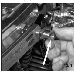
5. When using #71927 and a Mikuni 45mm, the vacuum fittings on the carburetor will not be accessible. The #71927 has a vacuum fitting to replace the blocked off carburetor vacuum sources and a plug that is to be used to plug the vacuum source on the carburetor.
