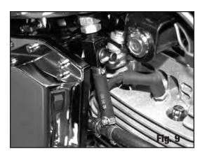
9. Connect nitrous hoses from nitrous plate to nitrous module assembly. Red to fuel solenoid and blue to nitrous solenoid. *(See Fig. 10).*
