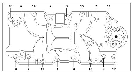
**Big Block Chevy Manifold Bolt Torque Sequence**
