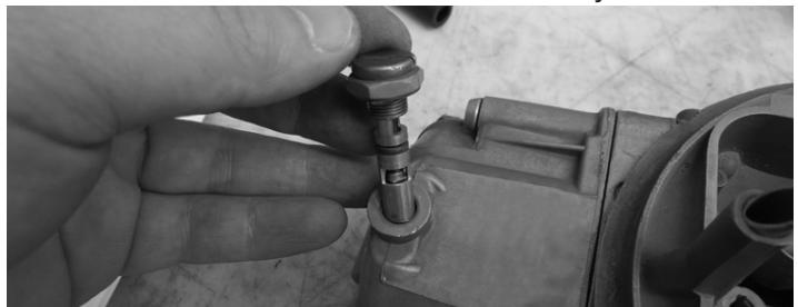
6. Using a flathead screwdriver, remove the idle mixture screws from the primary metering block, pull out the small cork O-rings and discard cork O-rings.
