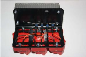
6: CHECK THAT WIRES DOESN'T MAKE CONTACT TO BRACKET OR BOLTS!
