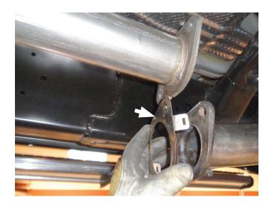
Secure each flange using bolt (3) through flat washer
