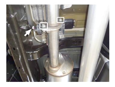
5. Remove muffler wire hangers from isolators, then remove muffler section from vehicle. Remove gasket from factory muffler inlet and retain for later re-use.
