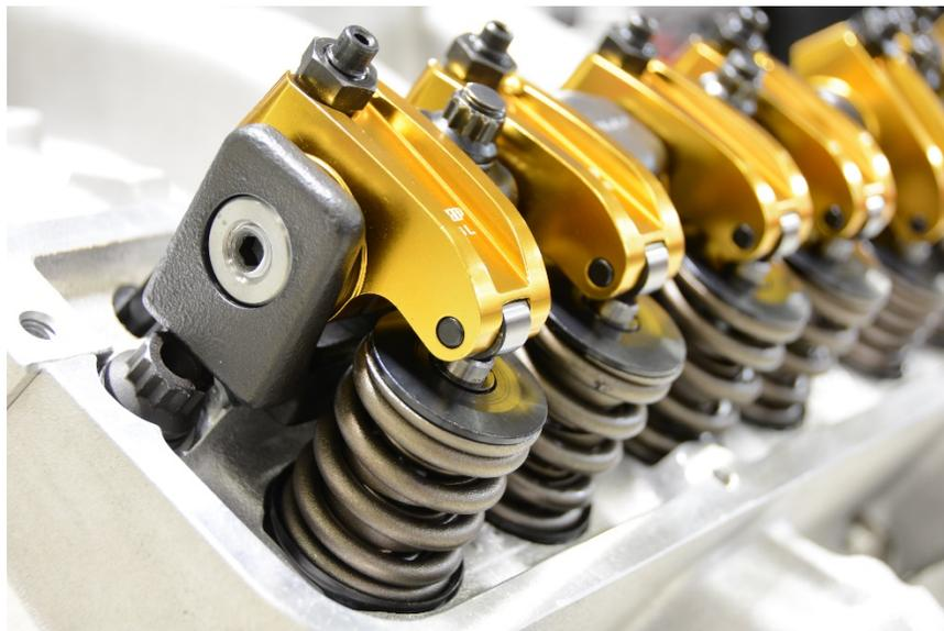
**Fig. 7 - Finished Rocker Assembly**
