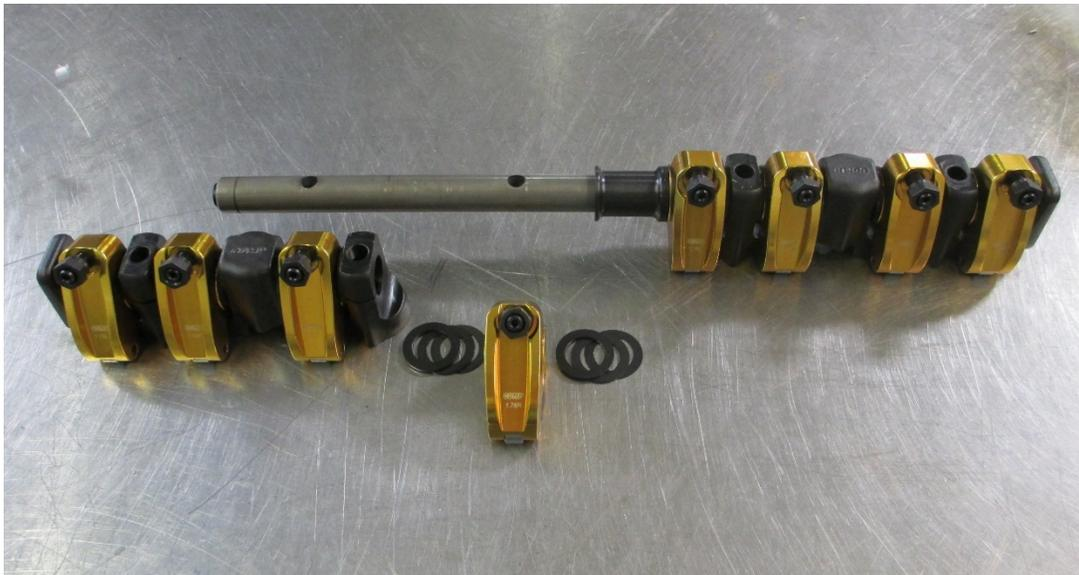
**Fig. 5 - Rocker Assembly with Rocker Removed and Spacers Shown**
