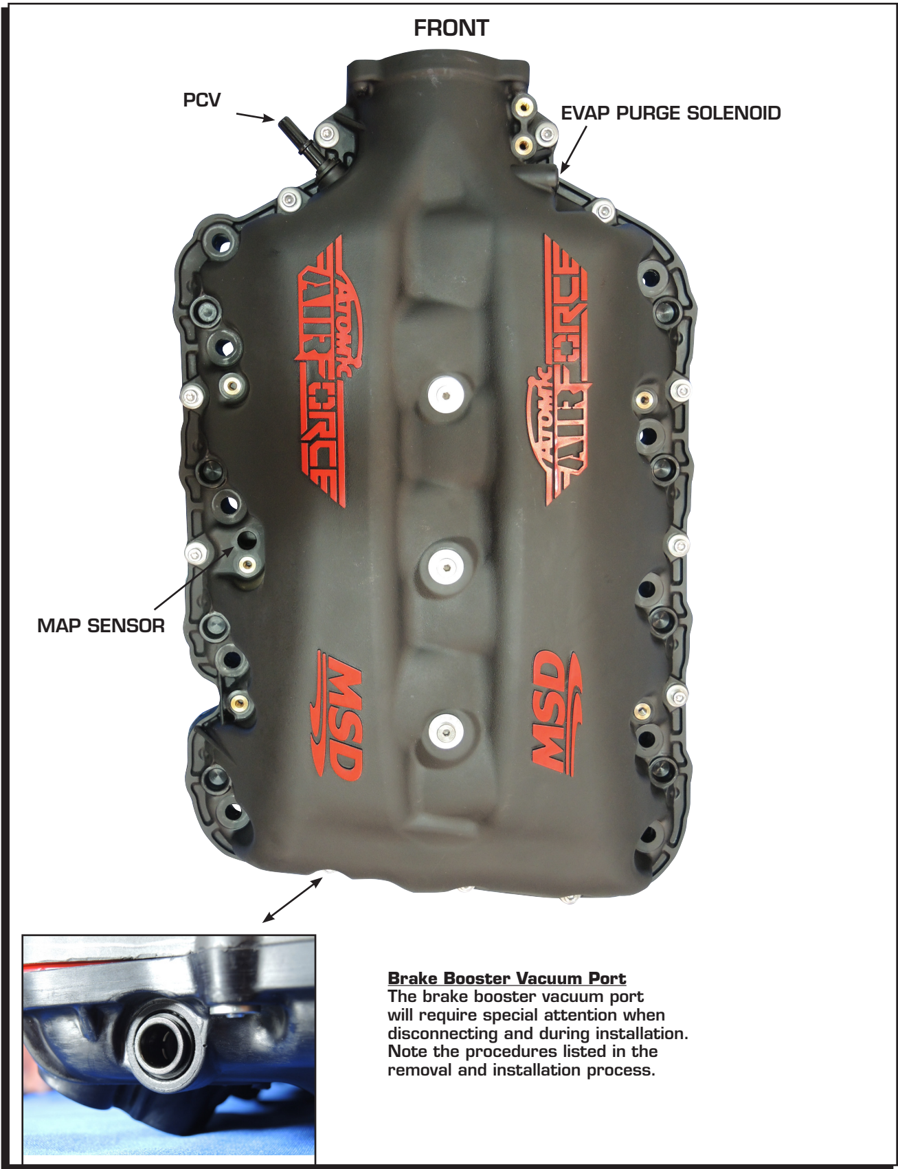
Figure 1 Vacuum Ports of the AirForce LT1 Manifold.
