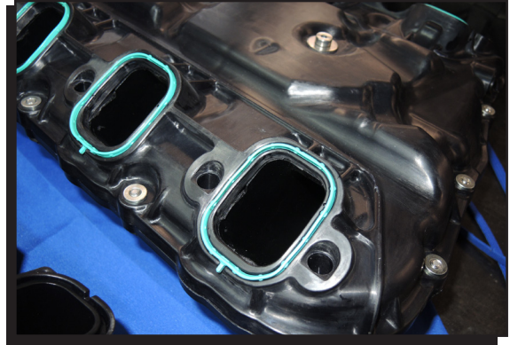
Figure 11 Install the Port Seals.
