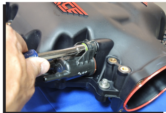
Figure 9 Install the EVAP Solenoid.
