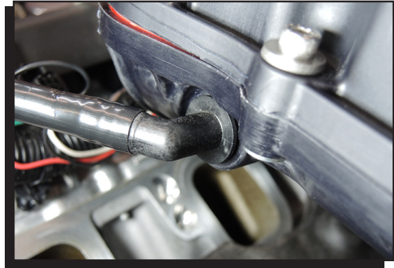
Figure 12 Connect the Brake Booster Tube.
