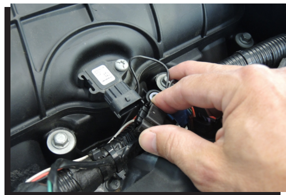
Figure 5 Disconnect the MAP Sensor.
