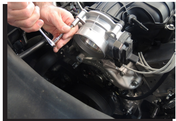
Figure 4 Remove the Throttle Body.
