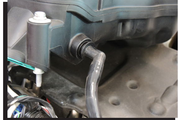
Figure 6 Brake Booster Vacuum Connection.
