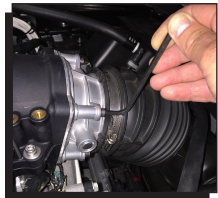
Figure 15 Installing the Throttle Body.
