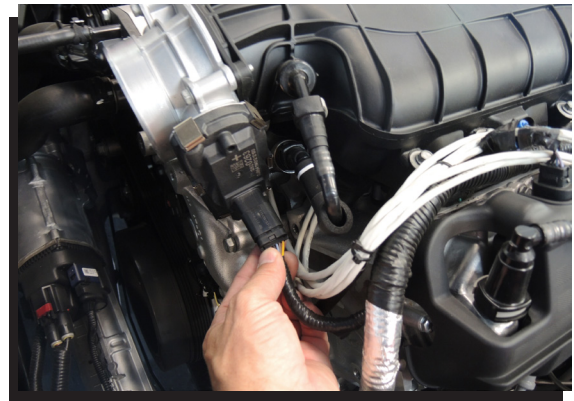
Figure 2 Disconnect the ETC.
