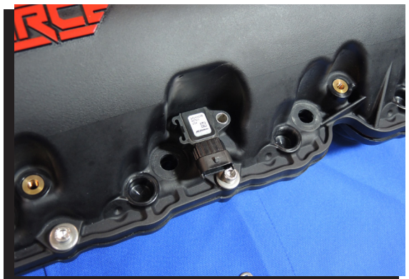
Figure 8 Install the MAP Sensor.
